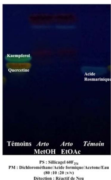
Figures 2. CCM chromatogram for phenolic acids from methanolic extracts (Arto MetOH) and ethyl acetate (Arto EtOAc) from Artocarpus heterophyllus at 366 nm.
