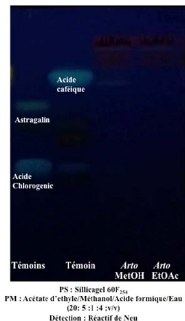
Figure 3. CCM chromatogram for flavonoids from methanolic extracts (Arto MetOH) and ethyl acetate (Arto EtOAc) from Artocarpus heterophyllus at 366 nm.
